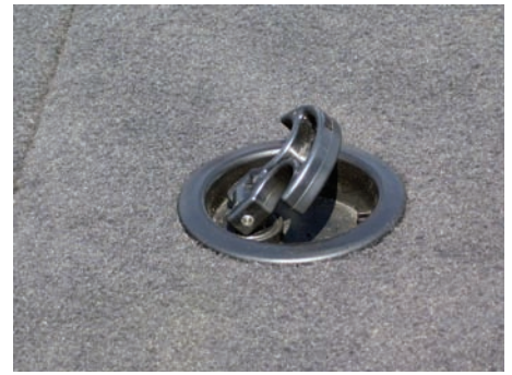
Left: A quick-release tie down with the passengers rods. Top Right: The livewell is fitted with a separator plate. Bottom Right: Hatch latches fold away and are easy to grasp.
