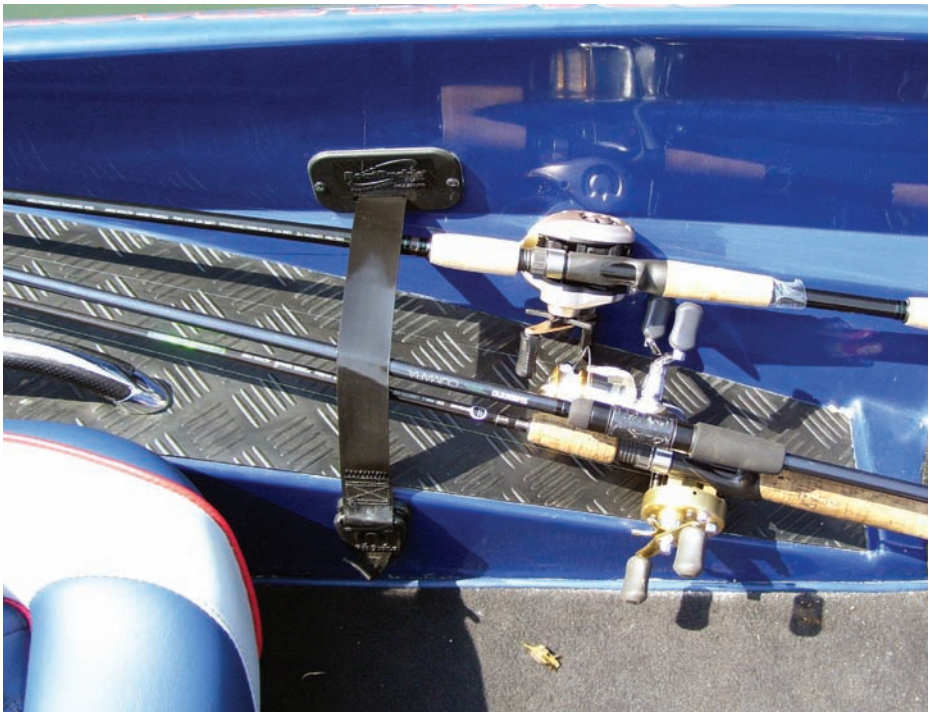
Left: A quick-release tie down with the passengers rods. Top Right: The livewell is fitted with a separator plate. Bottom Right: Hatch latches fold away and are easy to grasp.
